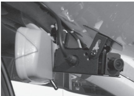
Fig. 8 Forward view camera box
