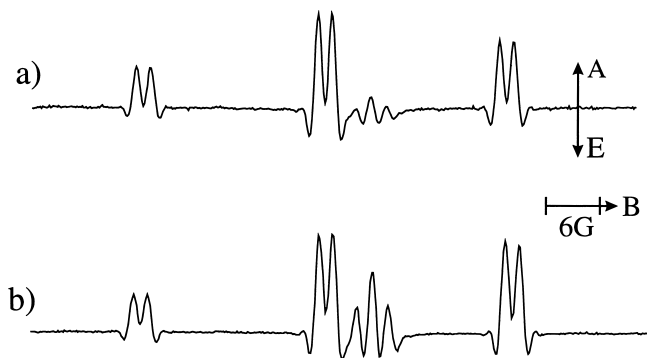
Fig. 2. Spectra observed a) in ethanol solution with \eta = 0.997 mPa s and b) in propan-1,2-diol solution with \eta = 30.28 mPa s. The fraction of radicals re-encountering would be expected to be higher in the high viscosity solution but even if it was unchanged the RPM contribution would be expected to grow by a factor of 5.5 relative to the TM one. This clearly is not the case, showing that the P_{TM} varies substantially with change of viscosity.
